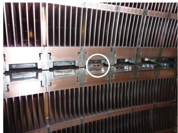
FIG. 7. (Color online) On the left picture is shown the 4 m reflectometry Ka waveguides located on top of the bottom half of the LH antenna launcher. On the right picture is a closer view of the reflectometer open waveguides facing the plasma in the middle of the full LH coupler.
