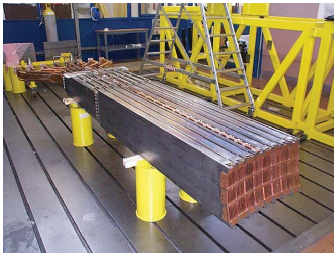
FIG. 7. (Color online) On the left picture is shown the 4 m reflectometry Ka waveguides located on top of the bottom half of the LH antenna launcher. On the right picture is a closer view of the reflectometer open waveguides facing the plasma in the middle of the full LH coupler.
