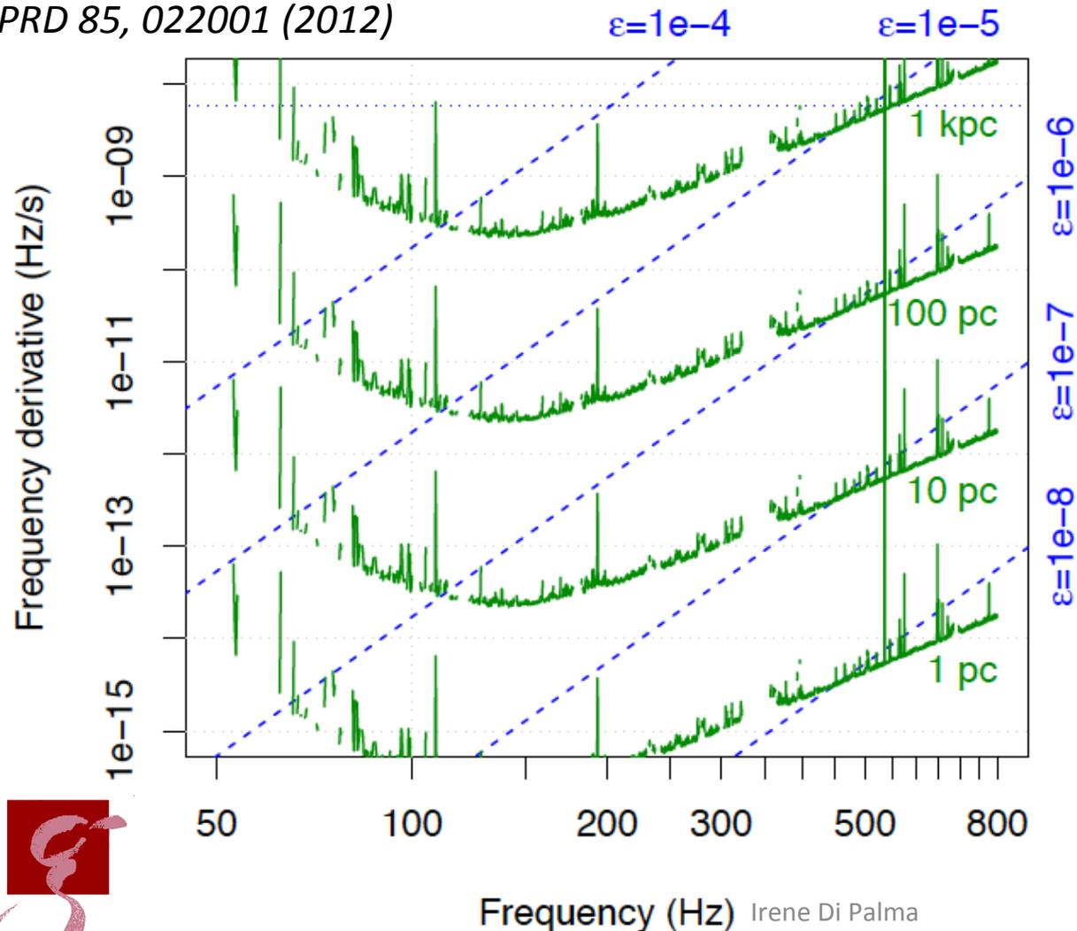
This is a superposition of two contour plots. The green solid lines are contours of the maximum distance at which a neutron star could be detected as a function of gravitational-wave frequency  $f$  and its derivative  $\dot{f}$ . The dashed lines are contours of the corresponding ellipticity ( $f$ ;  $\dot{f}$ ). The fine dotted line marks the maximum spin-down searched. Together these quantities tell us the maximum range of the search in terms of various populations.
