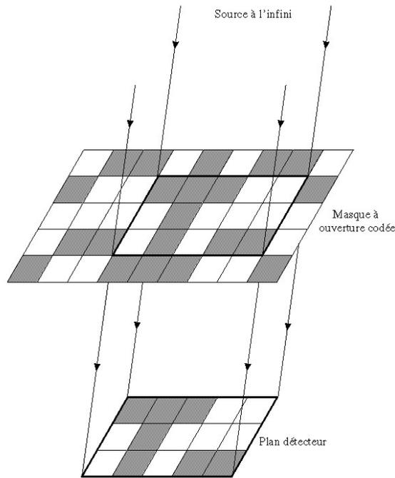
**Coded Aperture Systems** are based also on shielding. It employs a **mask** of opaque and transparent elements to modulate sky radiation before it is recorded by a **position sensitive detector**.
