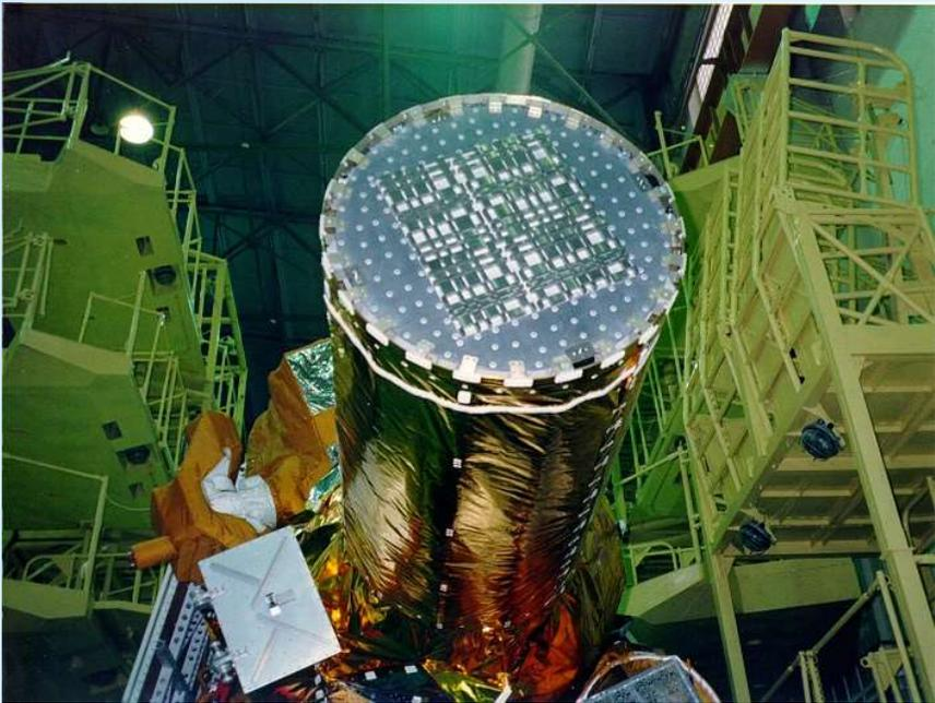
First gamma-ray space telescope with coded mask (URA)
