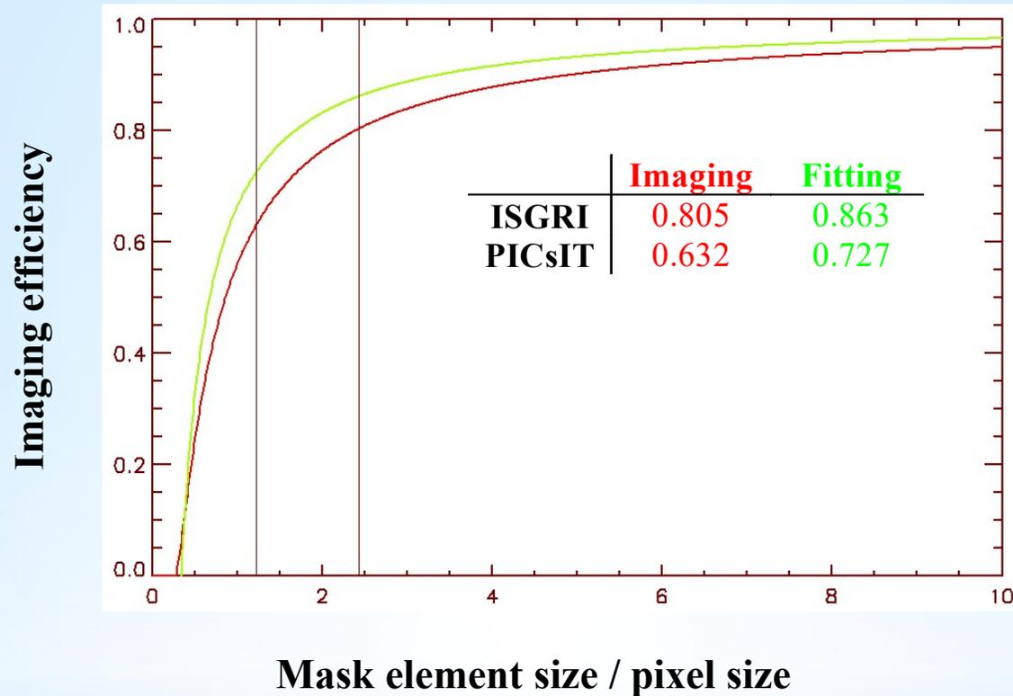
Expected average values of imaging efficiency due to discrete binning as function of the ratio ( $r$ ) between mask element – pixel sizes for simple fine cross-correlation and for SPSF fitting. Values expected for both IBIS detectors ISGRI ( $r=2.4$ ) and PICSIT ( $r=1.2$ ) pixel to mask element size ratios.
