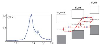
FIG. 4. (Color online) Left panel: critical current  $I_c^Q$  in units of  $e\Delta/\hbar$  as a function of the voltage in the quartet configuration, for resonant dots (same parameters as in Fig. 3). Right panel: lowest-order diagram contributing to the phase-dependent MAR current.
