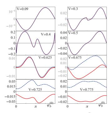
FIG. 3. (Color online) Current-phase relations  $I_a(\varphi_b^{(0)})$  (red, full curve) and  $I_b(\varphi_b^{(0)})$  (blue, dashed curve), in units of  $e\Delta/\hbar$ , in the quartet configuration  $V_a = -V_b$ , for the resonant dots regime:  $\varepsilon_a = -\varepsilon_b = 0.4\Delta$  and  $\Gamma = 0.1\Delta$ . Note the different y scales in the different panels.
