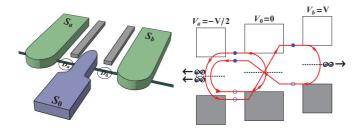
FIG. 1. (Color online) A Josephson bijunction (left). Superconductors  $S_{\alpha}$  ( $\alpha = a, b$ ) are biased at voltages  $V_{\alpha}$ , while  $S_0$  is grounded. The distance between the two quantum dot junctions is comparable to the coherence length. The right panel shows the energy diagram for the  $S_a D_a S_0 D_b S_b$  bijunction and a higher-order diagram associated with a "sextet" current with three pairs emitted, two in  $S_a$  and one in  $S_b$ , with  $V_a = -V_b/2$ .
