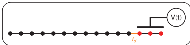
FIG. 1. (Color online) Sketch of the system: a tight-binding chain of length L , with a dot defined on one end (red sites, at the right of the t_d link), on which a time-dependent potential V(t) is applied.
