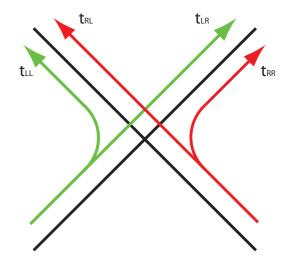
FIG. 2. (Color online) Reflectionless beam splitter with transition amplitudes.
