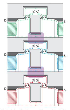
FIG. 5. (Color online) Geometry of the setup in the IQHE regime.  $S_j$  and  $S'_j$  (j = 1,2,3) are electron sources and  $D_j$  and  $D'_j$  are drains. Guiding centers of electron edge states meet at quantum point contacts, whose transparency can be controlled with gate voltages. The rounded rectangles indicate the interaction regions between neighboring MZIs. Space available for the Fermi sea is within the hatched regions.
