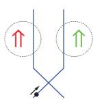
FIG. 4. (Color online) The three-MZI setup (up to lv2) represented in terms of spin counters: because of the interaction regions, the left and right MZIs in Fig. 1 act like spin counters (large arrows here) coupled to the left and right wires of the middle MZI.
