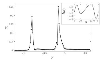
FIG. 8. SDE efficiency  $\eta_0$  for the quantum dot model of a Josephson diode in Appendix. We use units with  $\Delta=1$  and the parameters  $\alpha_0=1.4$ ,  $\mathbf{b}=(0.4,0,0.3)$ , L=3,  $t_L=0.45$ ,  $t_R=0.4$ , and  $k_BT=0.01$ . Main panel:  $\eta_0$  vs dot potential  $\mu$ . Lines connecting data points are a guide to the eye only. Inset: CPR for  $\mu=-0.16$ , where the SDE efficiency is  $\eta_0\approx0.25$ .
