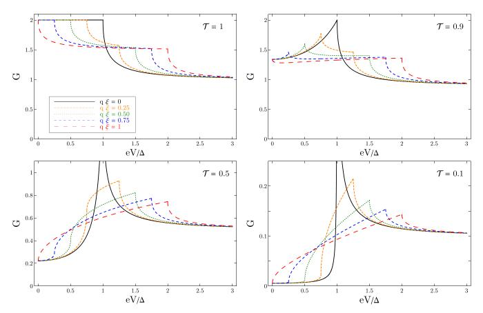
FIG. 3. Zero-temperature nonlinear conductance G(V) (in units of  $G_0 = 2e^2/h$ ) for a NS junction with several values for the CP momentum parameter  $q\xi$ . Since G(-V) = G(V), we only show G(V) for positive voltages. (a) is for transparency  $\mathcal{T} = 1$  and was obtained from Eq. (51). (b)–(d) are for  $\mathcal{T} = 0.9, 0.5, 0.1$ , respectively, and were obtained by numerically solving Eqs. (46) and (48).
