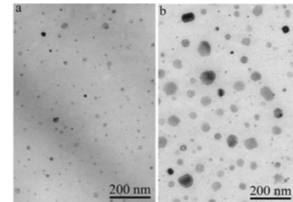
Fig. 1. TEM micrograph of annealed sample a) at 870 K for 780 h and b) at 1020 K for 3 h. Rounded metallic nano-particles enclose in the amorphous silicate. They formed by a reduction reaction and further precipitation since metallic Fe is immiscible in silicates. The microstructure closely resembles to those to GEMS found in IDPs.
