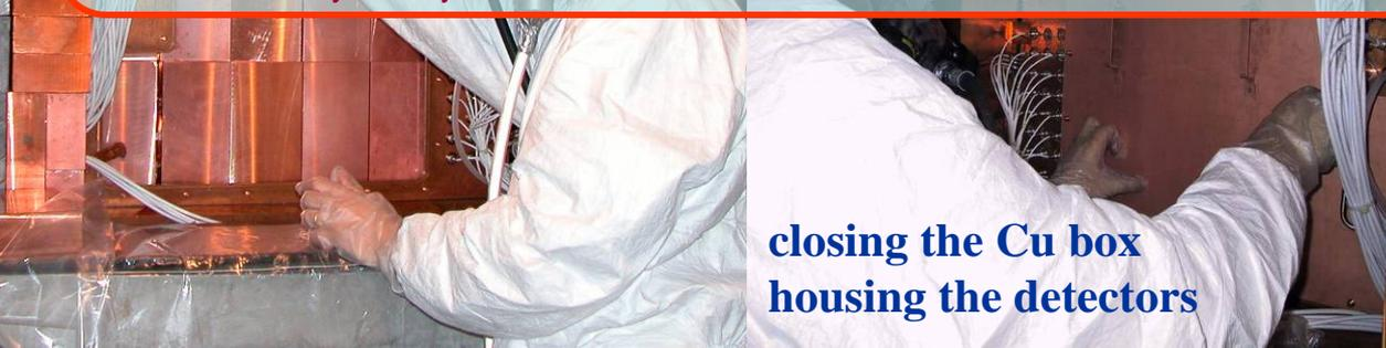
closing the Cu box housing the detectors
