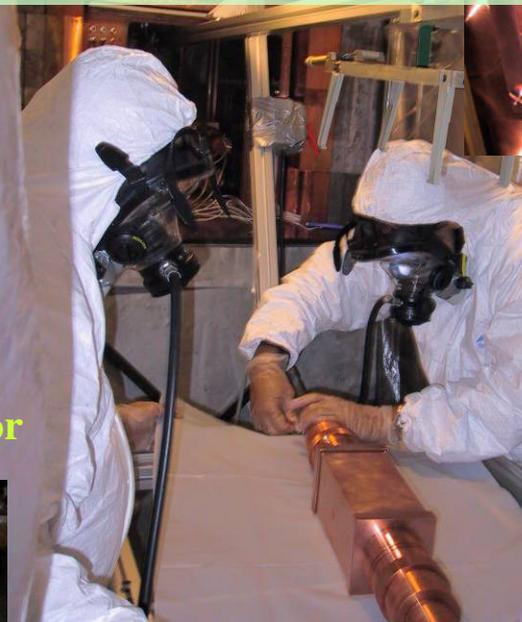
detectors during installation; in the central and right up detectors the new shaped Cu shield surrounding light guides (acting also as optical windows) and PMTs was not yet applied
