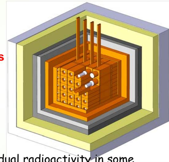
Residual radioactivity in some components of the DAMA/LIBRA passive shield (95% C.L.)
